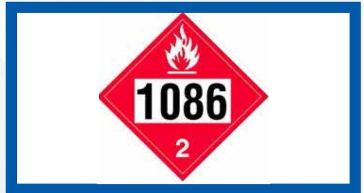
Responsibilities for marking and labelling the rail wagons or road tankers is very important. The labels can be painted or stencilled on the body of tank. Any old labels, signs & shunting labels which do not relate to the product to be transported or are damaged must be removed before shipment.
