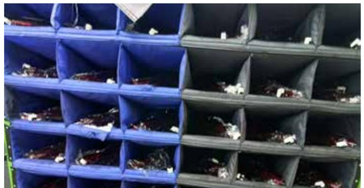
Pic-14 - Cushioned pigeon holes - for storage and transfer of production line fragile cargo (automobile industry)
