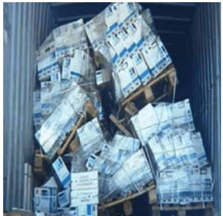
*Pic-22: Cargo loss due to improper securing*
