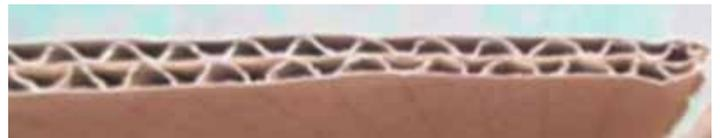
*Pic-5 side view of a "double-wall" (also called "5 ply wall"). As a general rule, a "single wall" is NOT suitable for export packing or for multiple handlings. A thicker wall will provide better protection, but it adds to total cost and to total volume.*
