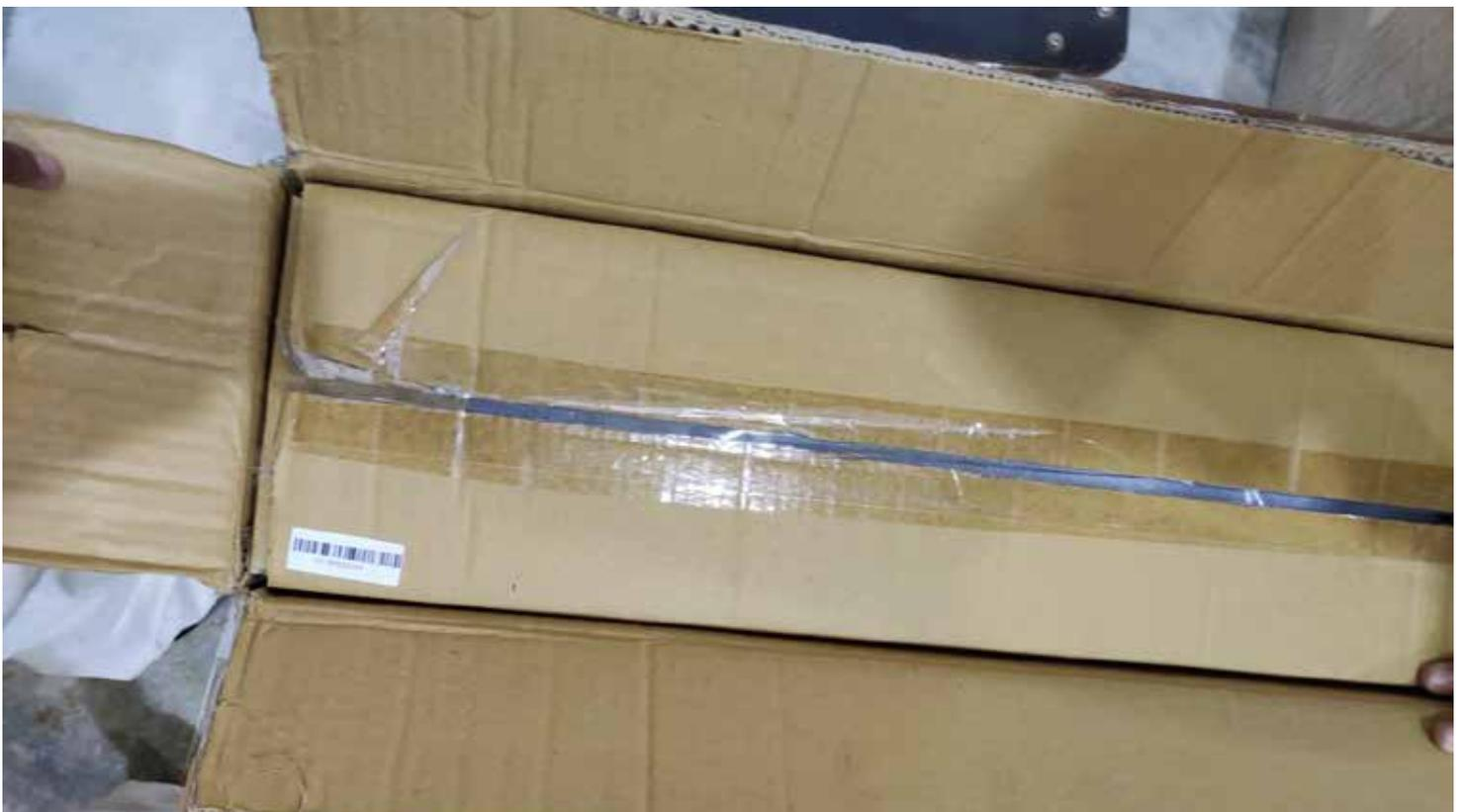
*Pic-24: Box in box packaging for electronics LCD Display*
