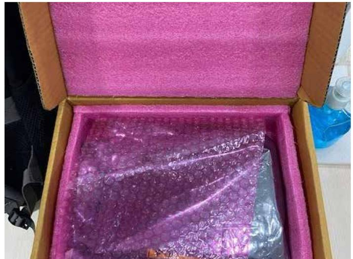
*Pic-8 Use of Foam Boards and bubble wrap*
