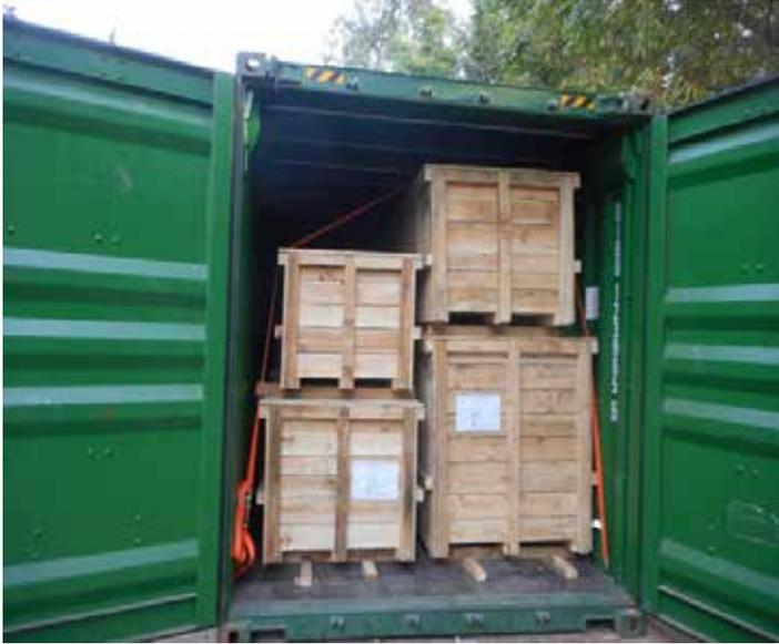
*Pic-19 and 20 – Proper securing of packages in transport and containers.*
