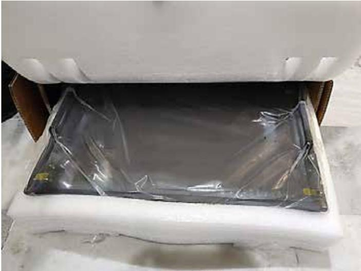
*Pic-21.1 – Packaging for LCD display – note the foam cushioning on either side.*
