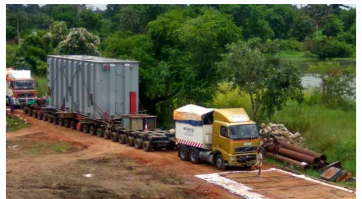
Hydraulic Multi -Axle Trailers with Puller – For Heavy loads more than 45 mt
