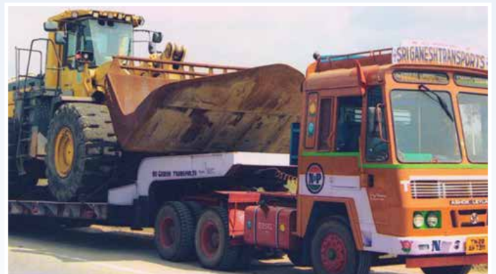
Semi Low bed trailers and Low bed trailers – Height more than 10 feet and 13 feet
