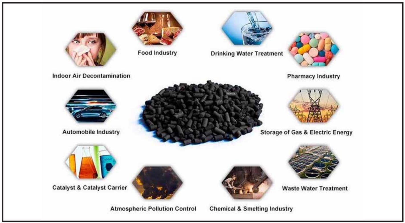
The properties of activated carbon allow it to remove undesirable impurities from a fluid. This works because carbon preferentially adsorbs the impurity onto its large internal surface within the pore structure. The pore sizes are usually characterised as follows:
