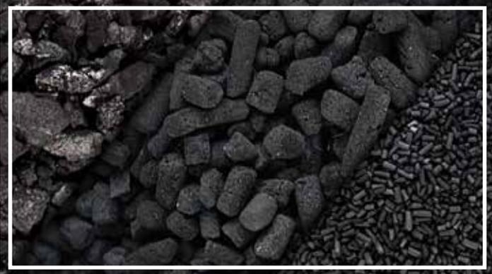
Activated carbons are produced and used as a black or dark grey solid, in granular, powder, pellet or textile form. It is produced from various types of raw materials such as bituminous coal, coconut shells, lignite, peat, synthetic sources, semi-anthracite and wood.
